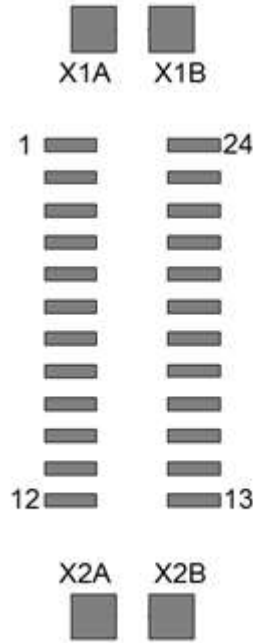
Figure 7: Pin Arrangement for E24 Interface
