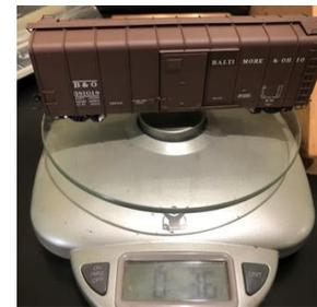
With the newer free rolling wheels and trucks today, exceeding the RP-20.1 recommendations is possible without creating excess drag. Many end users exceed this amount with good success. The values of RP-20.1 are the minimum recommended weights.
