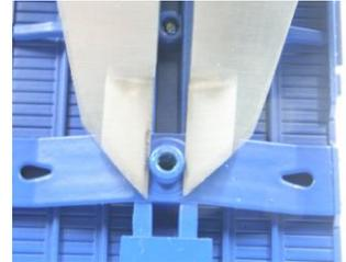
235 The inside of the truck bolster hole is easy to measure by using the inside jaws of the caliper. There is an offset that makes this measurement a bit more difficult. So, work the calipers around a bit to see that both jaws are against the inside of the bolster hole. The best performance is when the play between the kingpin and bolster is small without binding. Usually between 0.005”-0.010”
