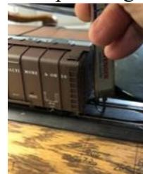
125 Care must be taken to not push down the coupler while taking this measurement. Employment of a re-rail track where the center of the re-rail track is at the same height as the top of rail can aid in taking these measurements. Both front and rear couplers shall be measured, and the values recorded.
